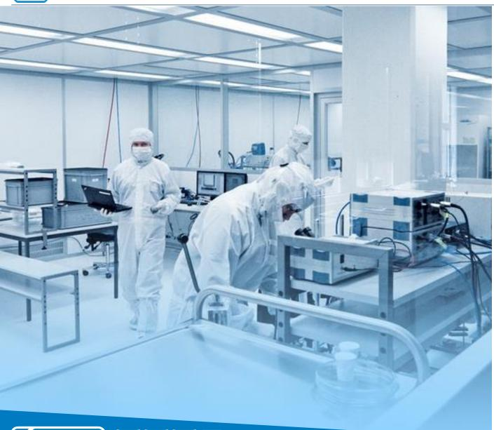
Controlled aera for manufacturing of components and goods that are sensitive to contamination.
